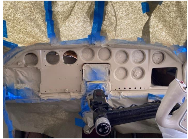
Previous Panel Hacks Repaired
